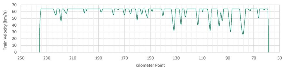
Figure 5-1: Train velocity for a freight train hauled by two Progress Rail Type 1 Battery Locomotives travelling south from Waskaganish (KP 236) to the lumber siding (KP 60)
