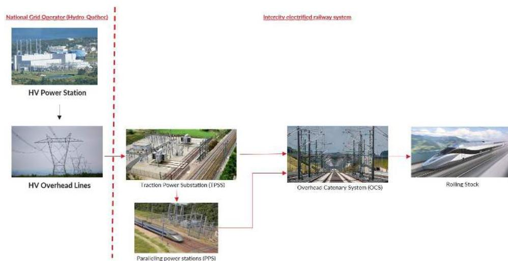
Figure 6-1: Schematic of the electrification infrastructure required
