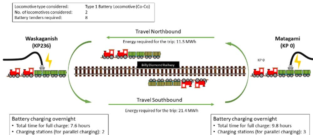
Figure 7-1: Train cycle diagram for Scenario B1
