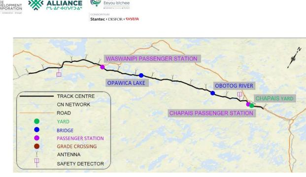
The line follows the existing subgrade both in plan and in profile. To avoid construction outside the existing right of way and to use the as many of the existing bridges as possible speed restriction are needed for approximately 11.5 km.
