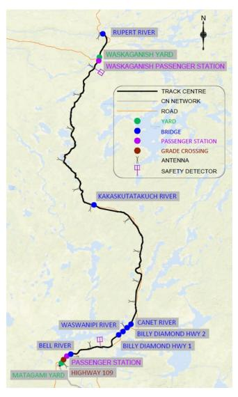
Much of the Billy Diamond Railway shares the same transportation route as the Billy Diamond Highway, using a corridor up to 100 m from the highway (60% of total alignment within 100m of the Billy Diamond Highway).
