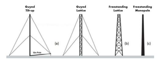
Figure 6-3: Typical Antenna Configurations
