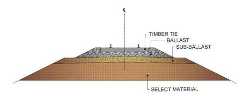
Figure 6-1: Standard Railroad Track Structure
