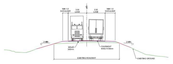
Figure 7-2 - Roadway cross section
