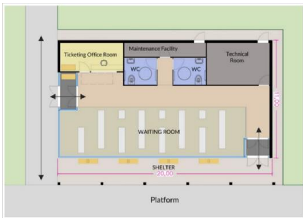
Figure 8.5-54: Layout of Station Building Rooms
