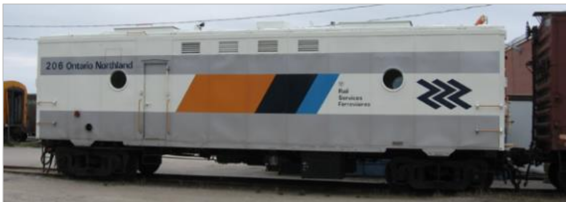
Figure 8.5-132: Typical Genset Car
