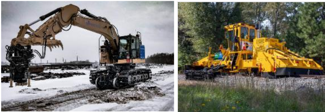
Figure 8.5-127: Railroad Excavator (Left), Ballast Regulator (Right)
