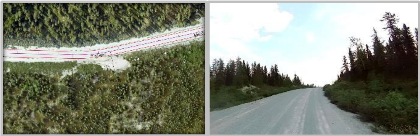
Figure 8.7-2: Street View July 2022 - Curve with radius too small at kilometer 69 (Route du Nord)
