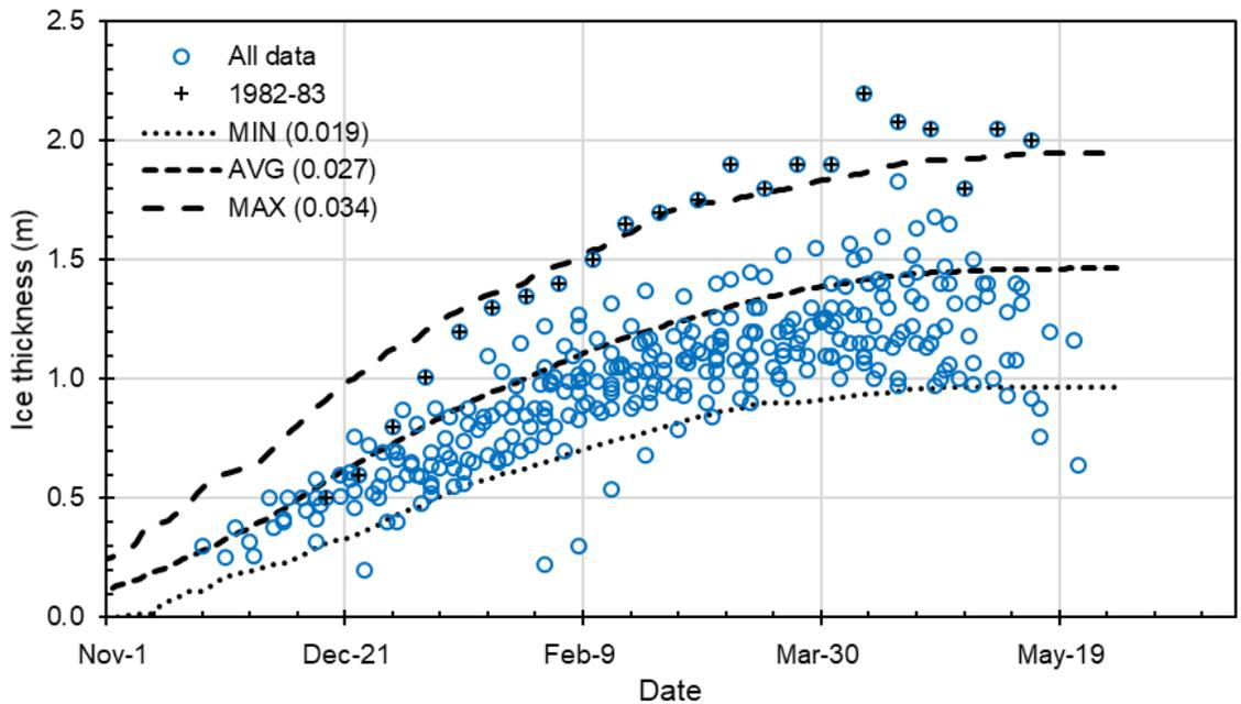
Figure 2-12 Ice thickness curves: Measured ice thickness between December 1972 (GC, blue circles) and 1982-83 (blue circles with black crosses), estimated curves based on Stefan equation with values 0.019, 0.027 and 0.034 m °C<sup>-1/2</sup> d<sup>-1/2</sup> (black dashed lines)
