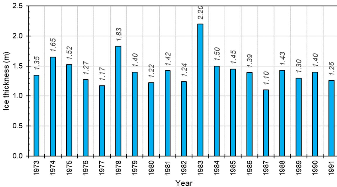
Figure 2-11 Maximum annual ice thickness measurement on the period 1973-1991. Based on measurements by the GC (2022)
